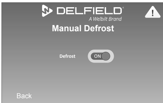
Settings Screen\Manual Defrost
